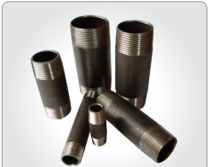
M.S Long Nipples & Close Nipples A105 SMLS, ERW SCH40, SCH80, SCH160 Size: 1/4" to 6" X 8" NPT & BSPT
