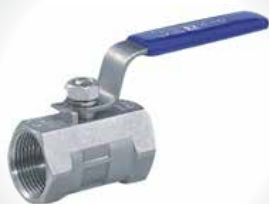
S.S. Ball Valve HEX Body R/B 1PC Body Design 1000WOG CF8M From 1/4" to 2" NPT
