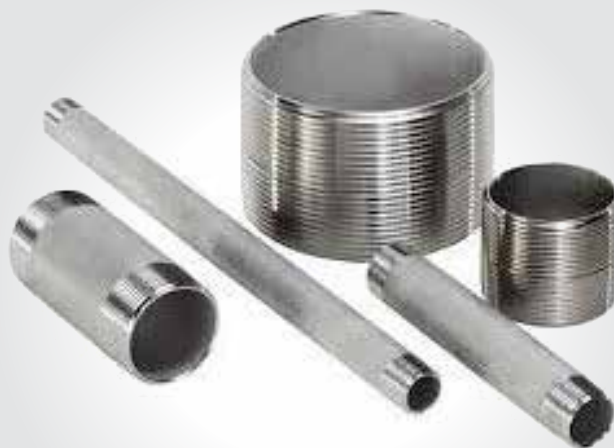
S.S Long Pipe Nipples & Close Nipples ERW & SMLS A182 316L SCH10, SCH40, SCH 80 From 1/4" to 4" x 6" Long 1/4" x 8" - 8" x 8" NPT & BSPT
